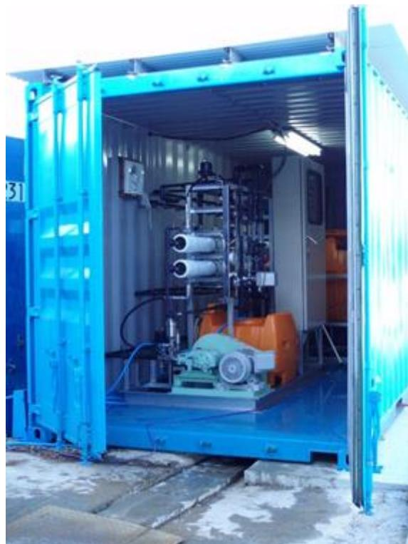
4)  $15 \text{ m}^3/\text{day}$  RO unit for seawater desalination (without sand filter)
