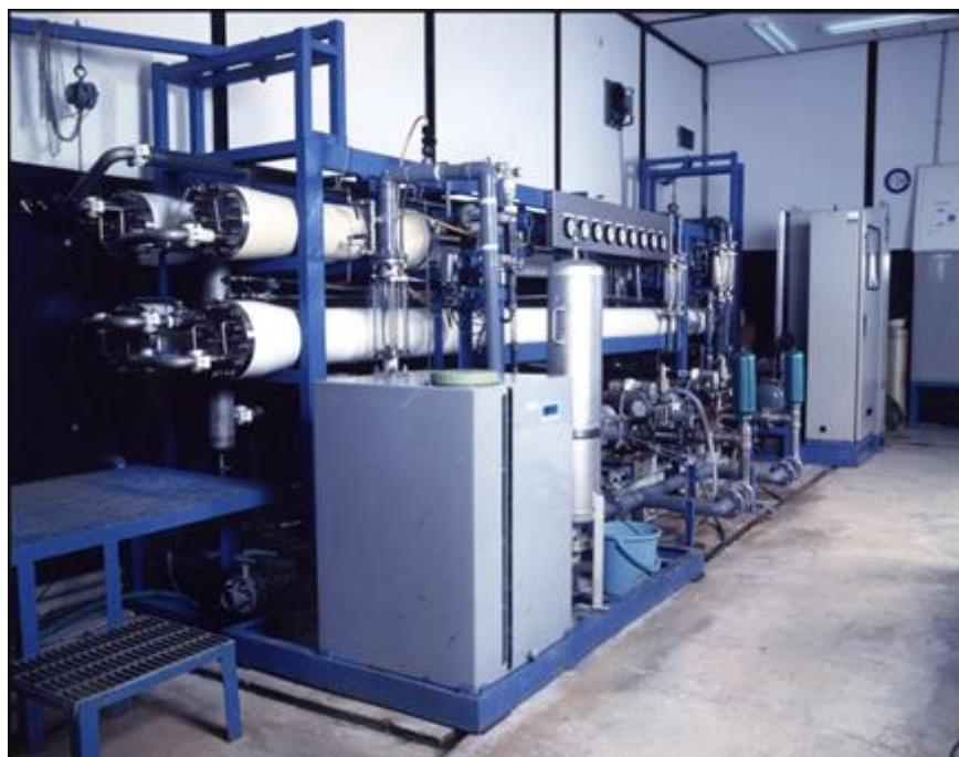
7)  $200 \text{ m}^3/\text{day} \times 2\text{sets}$  RO unit for seawater desalination
