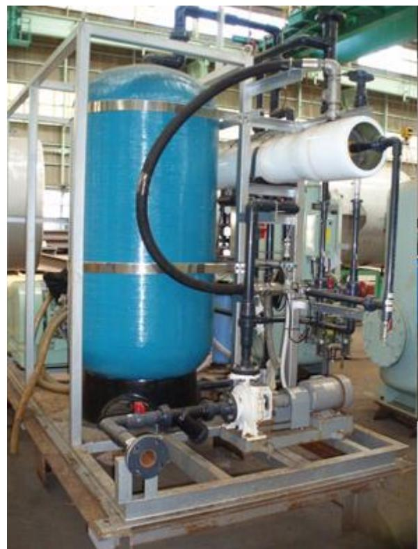
6)  $150 \text{ m}^3/\text{day} \times 2\text{sets}$  RO unit for seawater desalination
