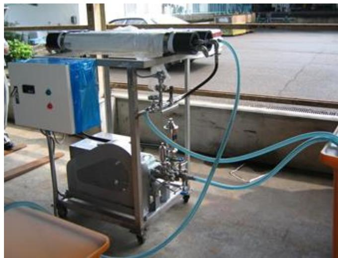
3)  $10 \text{ m}^3/\text{day}$  RO unit for seawater desalination
